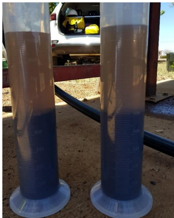
Figure 3-10: SVI testing for SVI1 (left) & SVI2 (right)
